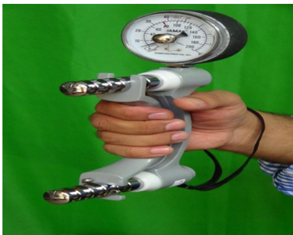
Figure 1: Hand-Held Dynamometer (Jammer)
